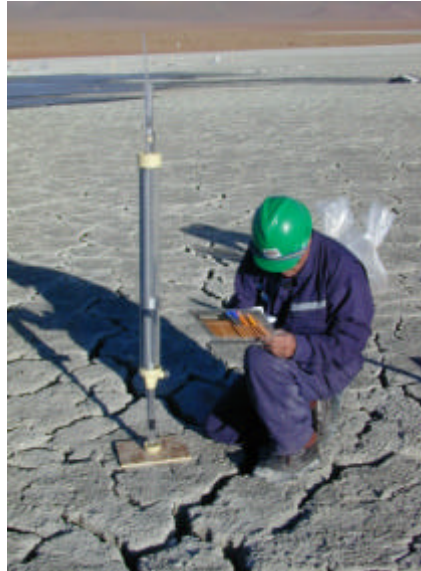
Photo 1: Guelph Permeameter testing in mine tailings, note dessication cracks at the surface (a courtesy of Robertson GeoConsultants Inc., 2003)
