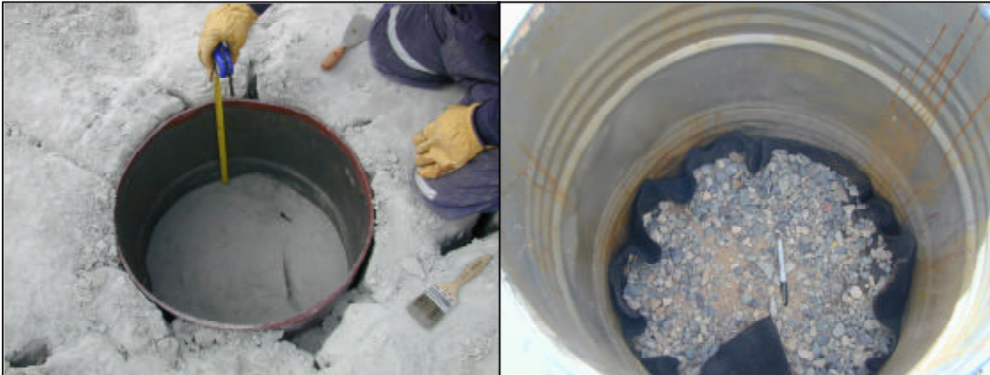
Photo 5a,b: Set up for single-ring infiltrometer test in mine tailings with “clean hole” base (a) and gravel-geofabric base (b) to simulate underdrain bottom condition (courtesy of Robsertson GeoConsultants Inc., 2003).
