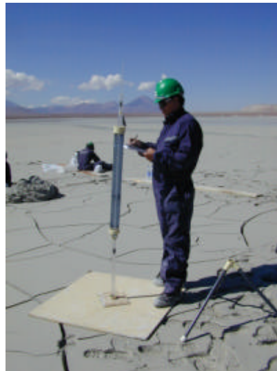
Photo 3: Set up for GP Testing in soft tailings using a wooden support platform (courtesy of Robertson GeoConsultants Inc., 2003)
