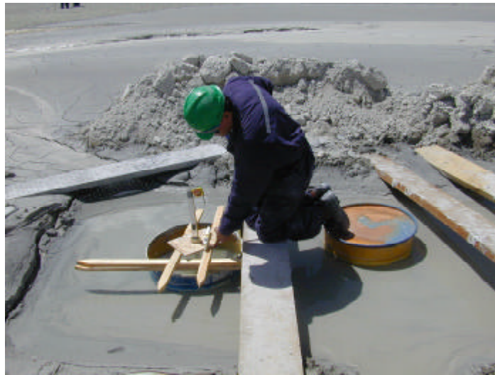
Photo 2: Set up for falling head testing in using the GP test tube in freshly deposited mine tailings (courtesy of Robertson GeoConsultants Inc., 2003).
